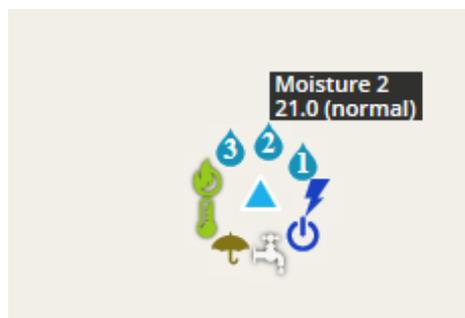
Figure 2. An schematic example of a reporting node at the Oregon State University, Malheur Experiment Station, Ontario, Oregon in 2016. The blue triangle indicates the node is reporting correctly while holding the mouse over each icon reports the current reading.
