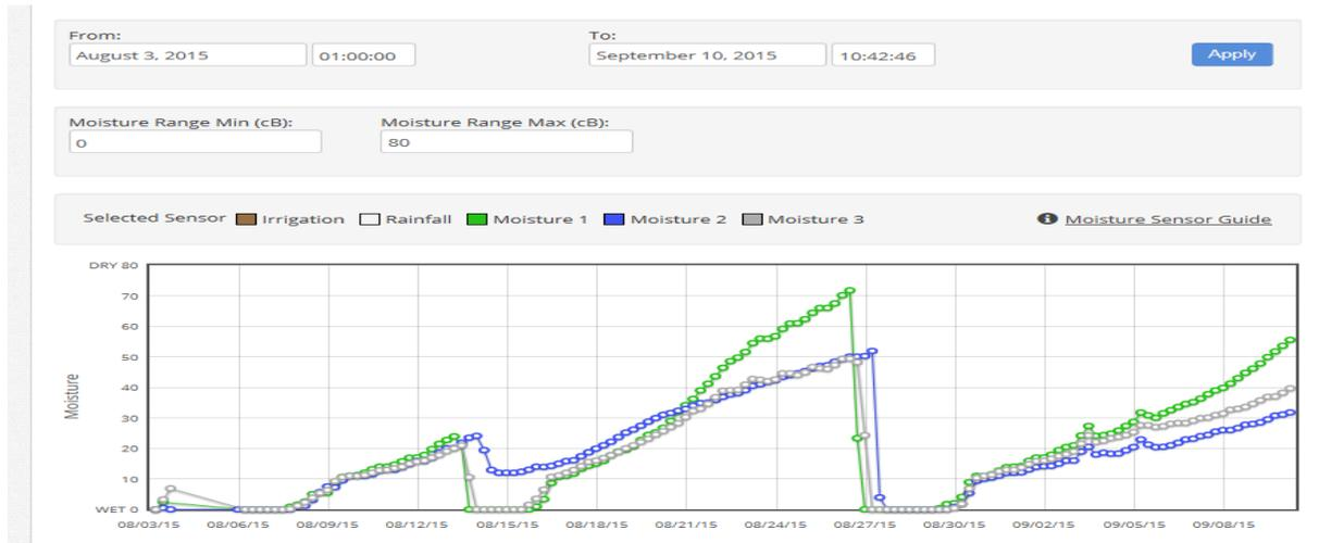
Figure 1. An example of a soil water tension records for three Watermark Soil Moisture Sensors at 8 inch depth in a furrow-irrigated quinoa field for a selected timeframe at the Oregon State University Malheur Experiment Station, Ontario, Oregon in 2015.
