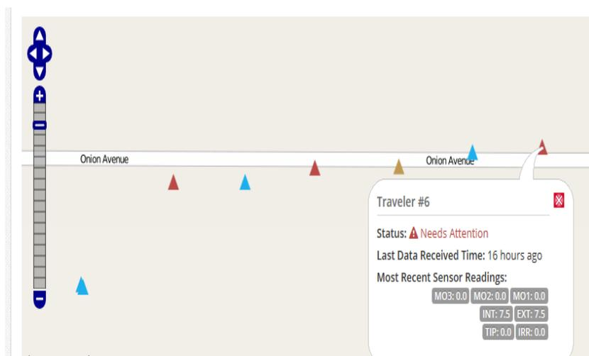
Figure 3. An schematic of a mesh deployment at the Oregon State University, Malheur Experiment Station, Ontario, Oregon. The blue indicates the node is reporting correctly, while the yellow icon indicates it has not reported recently. The red icon shows that it the node is not reporting at all.
