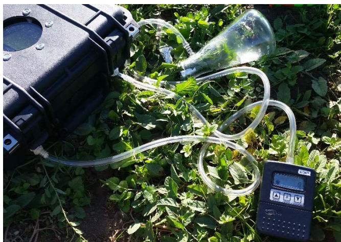
Figure 2 – Experimental setup to collect volatile compounds from bindweed. Insects use plant 'odors' as behavioral cues.
