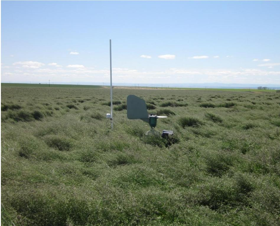
**Fig. 1.** A Burkard volumetric 7-day recording spore trap and weather data logger deployed in a commercial Kentucky bluegrass seed production field.
